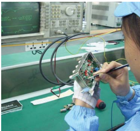
Every unit is carefully tuned and tested individually using a network analyzer.
